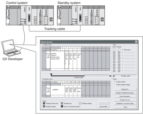
Diagram 1.12 System Monitor of GX Developer
