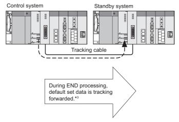
Diagram 5.47 Data Transfer by Tracking Function
