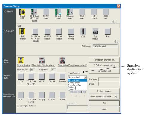
**Diagram 6.1 Connection Setup Window**
