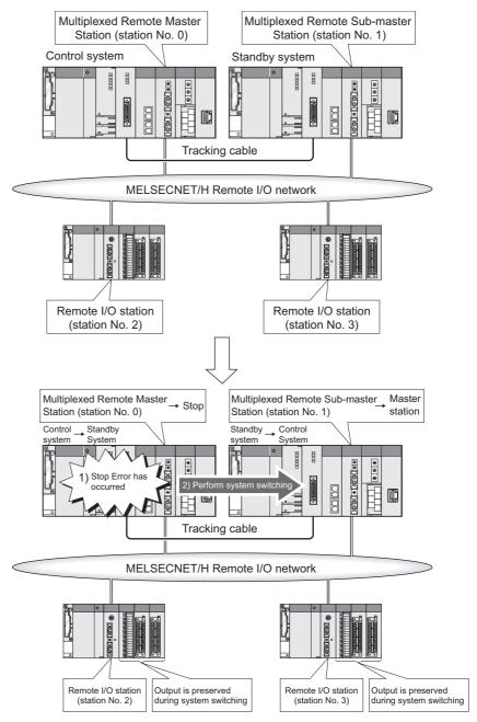
Diagram 6.14 Redundant System Operation at System Switching
