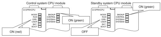
Diagram 5.89 LED Indications during Standby System CPU Module Operation
