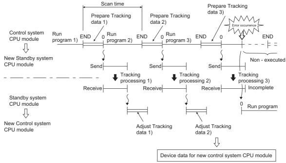
Diagram 5.55 Tracking Operation Timing When Program Execution Time ≥ Tracking Processing Time
