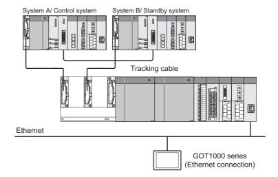
Diagram 6.49 GOT Connection Type (when Mounting to Extension Base Unit)
