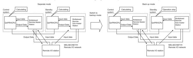
Diagram 5.46 Operations When Changing from Separate Mode to Backup Mode
