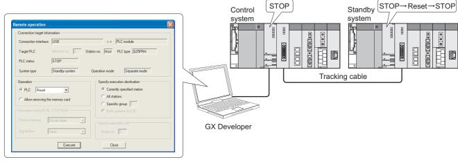
Diagram 5.103 Remote Reset Operation in Separate Mode
