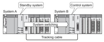
Diagram App.27 The system when System B is switched to the control system through a system switching instruction
