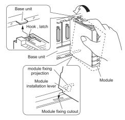
**Diagram 4.3 Procedure for Mounting Modules**
