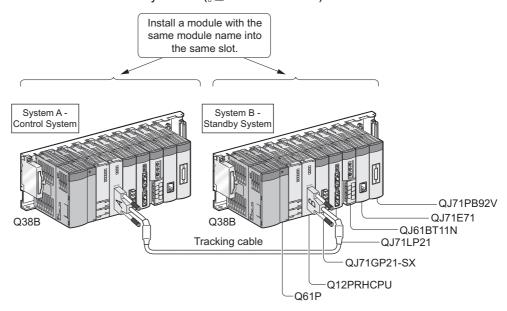
**Diagram 2.2 Redundant System Configuration**
