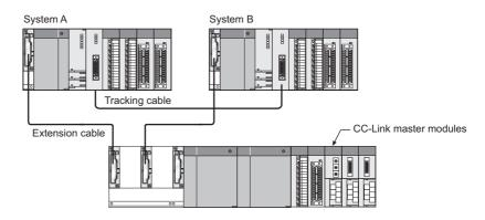
Diagram App.30 System configuration when CC-Link master module is mounted on the extension base unit
