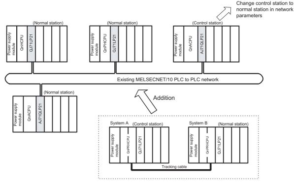
Diagram 6.12 Changing the Control Station When Adding Redundant System
