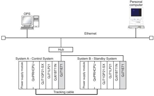
Diagram 2.4 Connection of Redundant System to Ethernet
