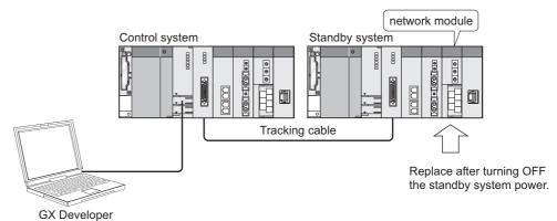
Diagram 8.30 System where Standby System Network Module Is Replaced
