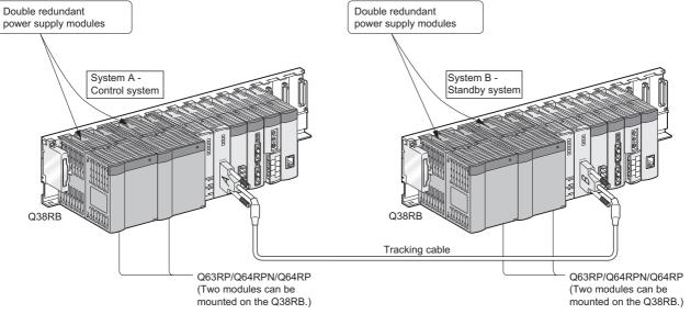
Diagram 2.3 Power Supply Modules and Redundant System
