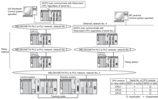
Diagram 6.50 System Configuration for Communication from Other Networks with "Control System" Specified
