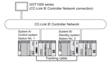
Diagram 6.47 GOT Connection Method (CC-Link IE Controller Network)
