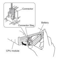
Diagram 4.6 Connecting the Case Connector and Battery Connector Pin
