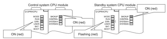
Diagram 5.83 LED Indications at Memory Copy Completion
