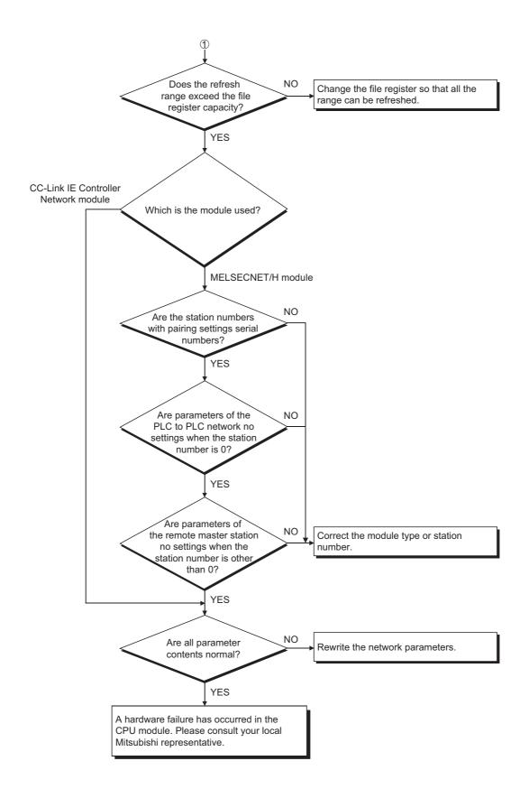
Diagram 8.15 Flowchart for when "LINK PARA. ERROR" Occurs
