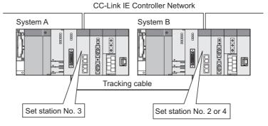
Diagram 6.10 Station No. settings for the network module
