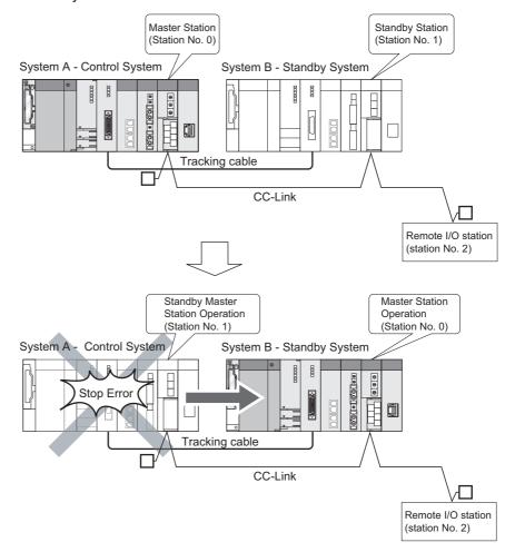
Diagram 6.35 Operation at System Switching due to Control System Error
