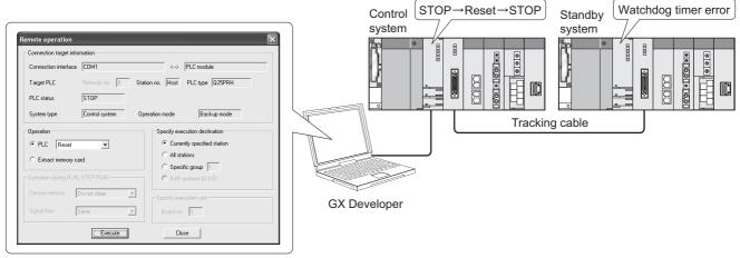
Diagram 5.105 Remote Reset Operation When Watchdog Timer Error Has Occurred in Standby System CPU Module
