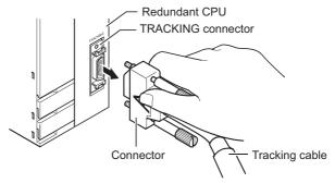
**Diagram 3.6 Disconnecting the Tracking Cable**
