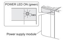
Diagram 4.9 Confirm that the "POWER" LED of power supply module is ON
