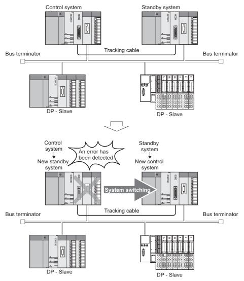
Diagram 1.6 System Configuration for PROFIBUS-DP
