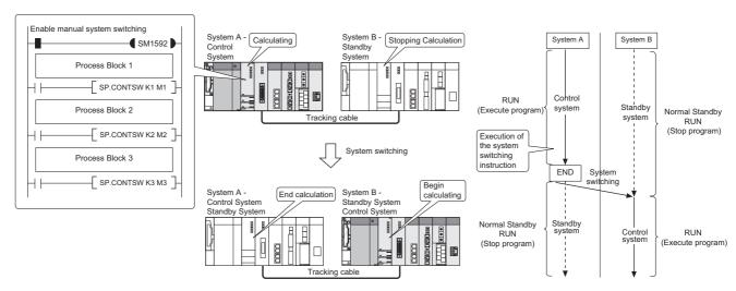
Diagram 5.28 System Switching Operation by System Switching Instruction
