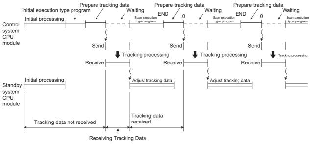
Diagram 5.58 Tracking Operation Timing in Program Synchronized Mode
