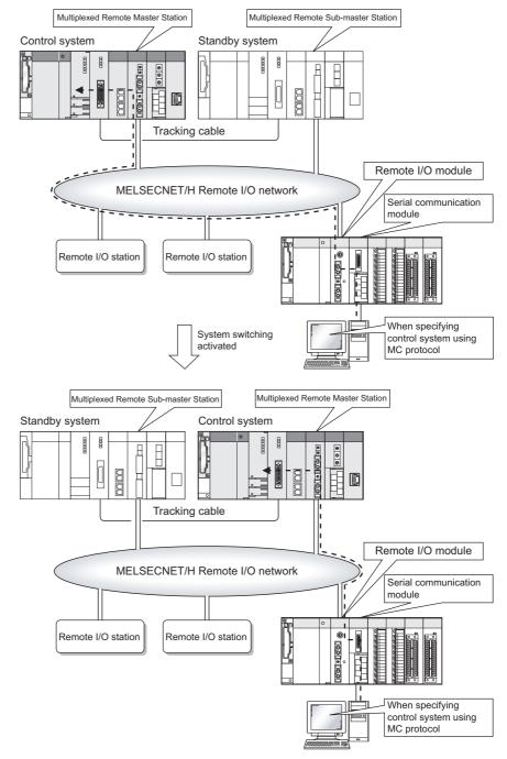
Diagram 6.40 Operation for Communication with Control System CPU Module by MC Protocol
