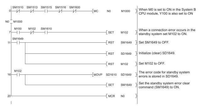
Diagram 8.18 Sample Program for Clearing Standby System CPU Module Error
