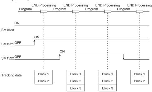
Diagram 5.50 Tracking Operation Timing by Tracking Trigger
