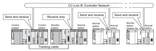
Diagram 6.7 Communication between Control System and Standby System Network Modules
