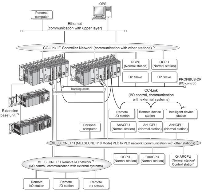
Diagram 2.1 Example of Redundant System Configuration
