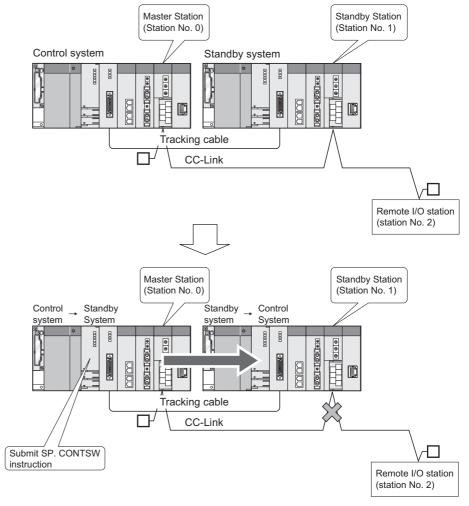
Diagram 6.37 Operation When System Switching Is Manually Carried Out
