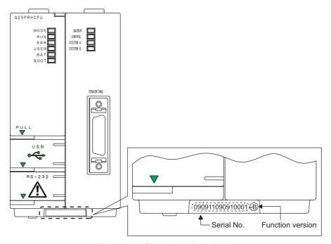
Diagram 2.13 CPU module front display
