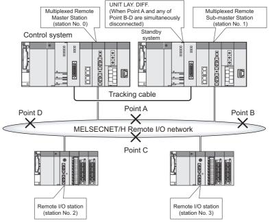
**Diagram 6.18 Error Detection at Cable Disconnection**
