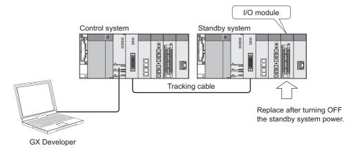
Diagram 8.26 I/O Module Replacement System during Power OFF
