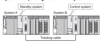
Diagram App.24 The system when System B is operating as the control system
