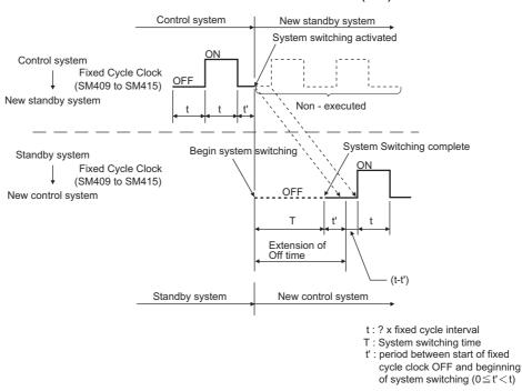
Diagram 7.6 Operations of Fixed-scan Clocks at System Switching
