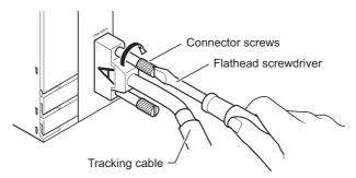
Diagram 3.4 Fixing the Tracking cable Connector
