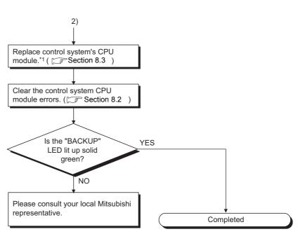
Diagram 8.4 Flow for the Case where the CPU Module BACKUP LED is ON (Lit Red)
