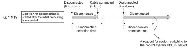
Diagram 6.28 System Switching Timing at Disconnection Detection
