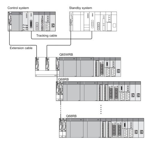
Diagram 1.3 System Configuration when Connecting Extension Base Unit
