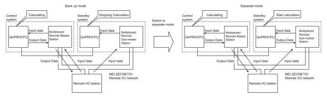
Diagram 5.45 Operations When Changing from Backup Mode to Separate Mode
