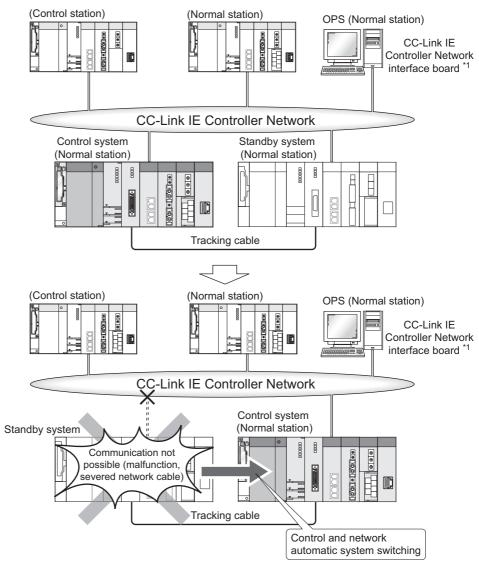
Diagram 1.4 System Configuration for CC-Link IE Controller Network
