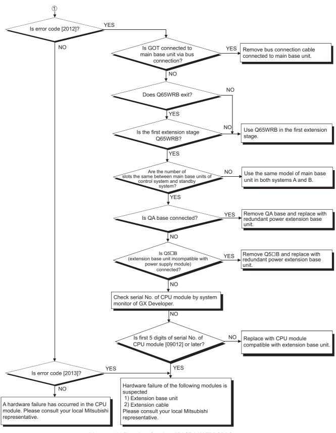
Diagram 8.11 Flowchart for when "BASE LAY ERROR" Occurs
