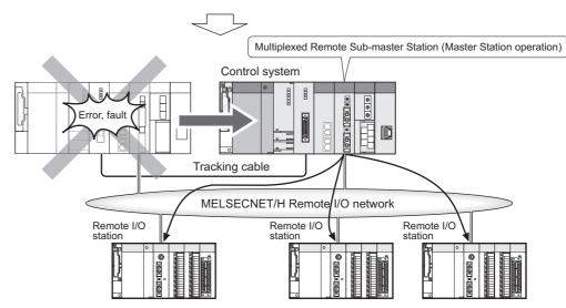
Diagram 1.5 System Configuration for MELSECNET/H Remote I/O Network
