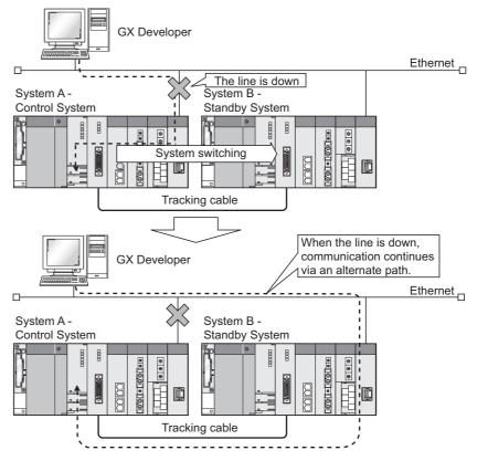
Diagram 6.5 Communication continuation through system switching
