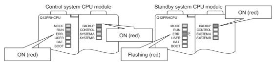
Diagram 5.88 LED Indications at Memory Copy Completion
