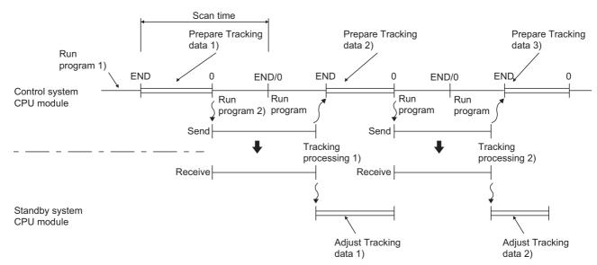
Diagram 5.56 Tracking Operation Timing When Program Execution Time < Tracking Processing Time
