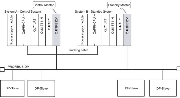
Diagram 2.10 Connection of Redundant System to PROFIBUS-DP
