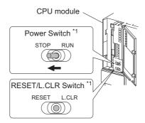
Diagram 4.8 CPU Module Switch Positions and Settings
