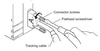
Diagram 3.5 How to Loosen the Connector Fixing Screws
