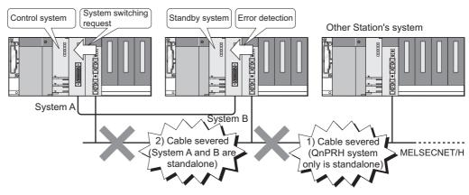
Diagram 5.25 System Switching Operation at Cable Disconnection
