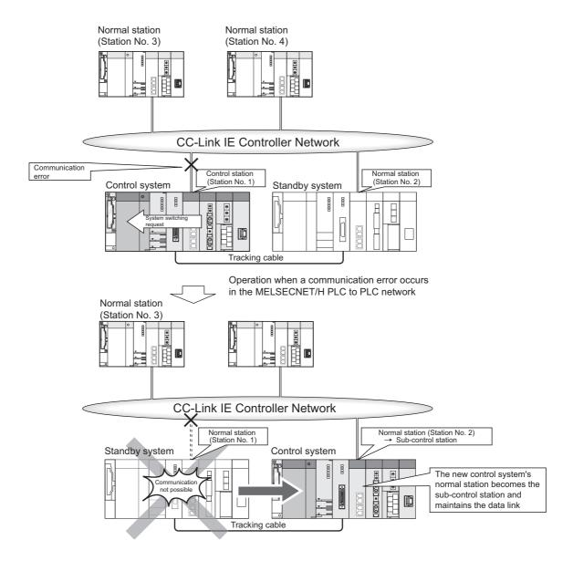
Diagram 6.9 Continuation of Data Link via System Switching
