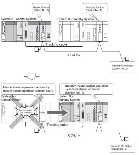
Diagram 6.33 CC-Link Operation at System Switching
