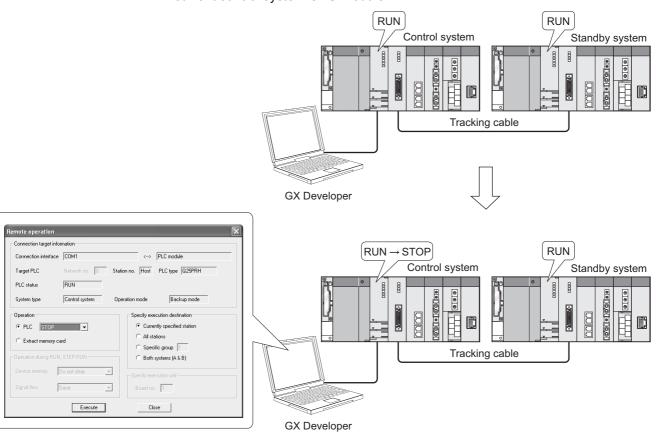
Diagram 5.99 Remote STOP Operation When Current Station Is Specified
