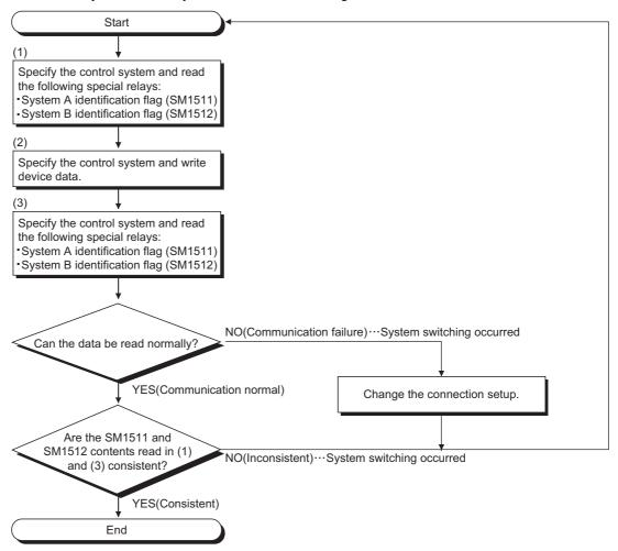
Diagram 6.52 Flowchart for Checking for System Switching with the system A and system B identification Flags
