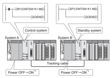
Diagram App.26 The system when both systems are simultaneously powered ON
