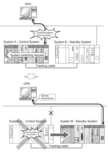
**Diagram 6.22 Operation at Communication Error Detection**
