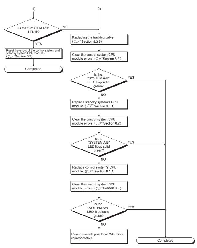
Diagram 8.5 Flow for the Case where the SYSTEM A/B LED is Flashing
