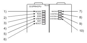
**Diagram 8.1 CPU Module LEDs**
