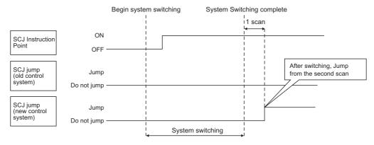
Diagram 7.3 ON/OFF Operation of SCJ Instruction When Signal Flow Has Been Tracked
