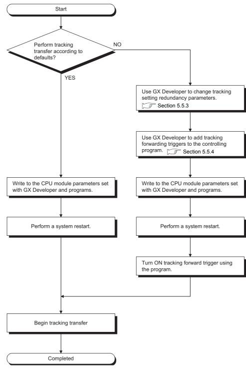
**Diagram 5.48 Tracking Execution Procedure**
