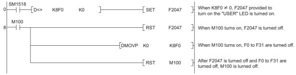
Diagram 7.13 Program That Turns on the "USER" LED after System Switching
