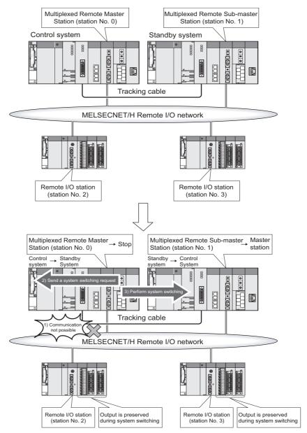
Diagram 6.15 Output Status during System Switching
