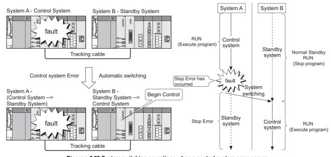
Diagram 5.23 System switching operations when a control system error occurs
