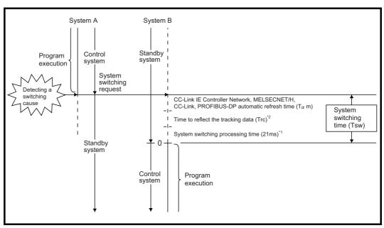
**Diagram 9.1 System Switching Timing**
