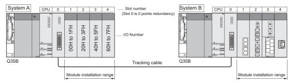
Diagram 2.15 Number of Slots Occupied by Redundant CPU and I/O Numbers of Main Base Units
