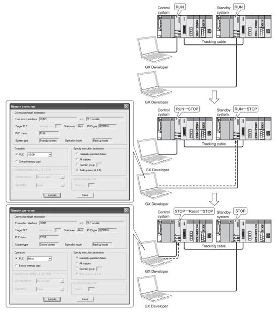
Diagram 5.106 Remote Reset Operation after Execution of Remote STOP for Control System or Standby System CPU Module from Other Route
