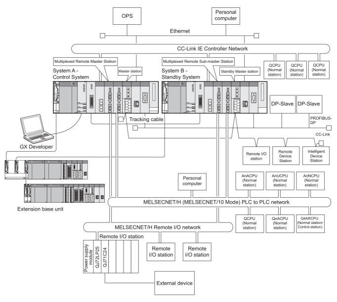
Diagram 6.6 Redundant System Network
