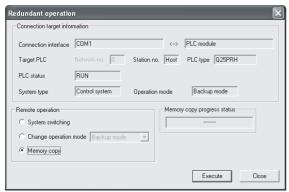
Diagram 5.77 Redundant Operation Window Showing Normal Completion
