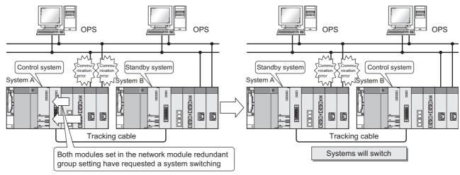
Diagram 5.93 Operation When Error Occurs on Both Networks
