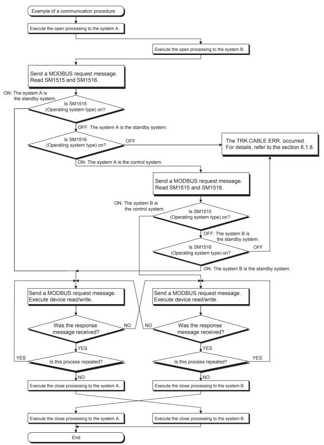
Diagram 6.31 Communication Example for Fixed IP Mode
