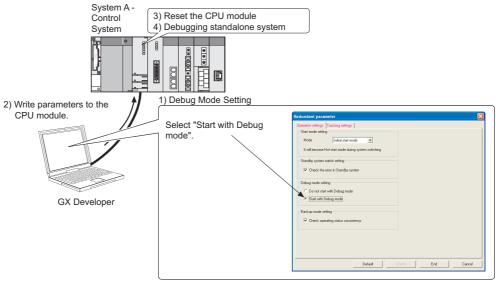
Diagram 5.9 Setting of Debug Mode on Redundant Parameter Window
