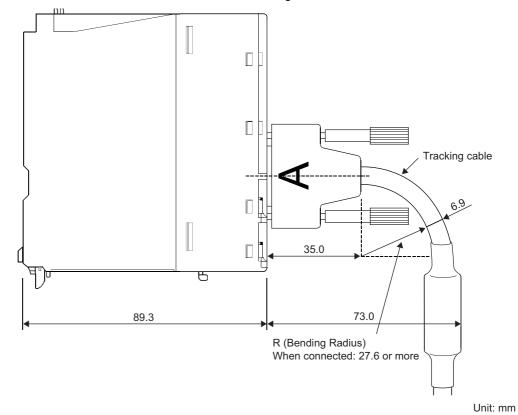
Diagram 3.1 Minimum Bending Radius of a Tracking Cable
