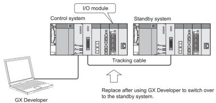
Diagram 8.27 I/O Module Replacement System during Power ON
