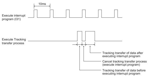
Diagram 7.10 Operations When Interrupt Is Executed by Internal Timer
