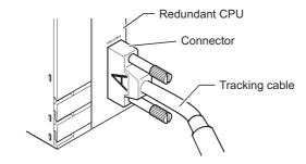
Diagram 3.3 Connecting the Tracking cable Connector
