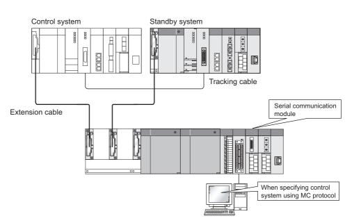
Diagram 6.39 Operation for Communication with Control System CPU Module by MC Protocol
