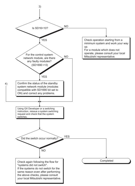
Diagram 8.9 Flow in the Case of System Switching due to Control System Error or System Switching Instruction Execution
