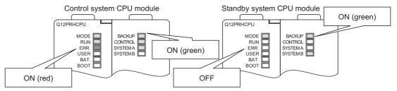
Diagram 5.84 LED Indications during Standby System CPU Module Operation
