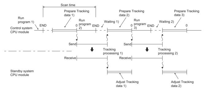
Diagram 5.54 Tracking Operation Timing When Program Execution Time < Tracking Processing Time
