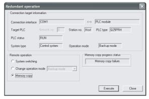
Diagram 5.78 Redundant Operation Window Showing Abnormal Completion
