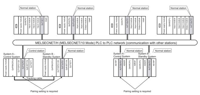
Diagram 2.5 Connection of Redundant System to MELSECNET/H PLC to PLC Network
