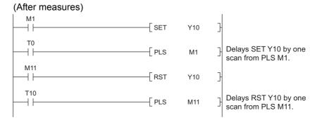
Diagram 7.20 Program Example when Outputting by timer contact
