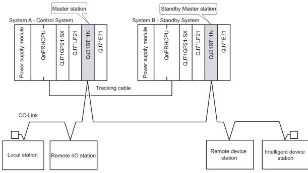
Diagram 2.8 Connection of Redundant System to CC-Link
