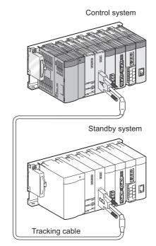
Diagram 1.14 Vertical Arrangement of Control System and Standby System
