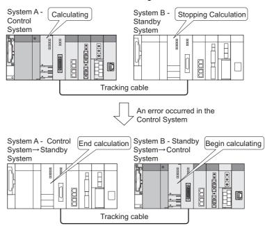
Diagram 5.8 System Switching Operation in Backup Mode
