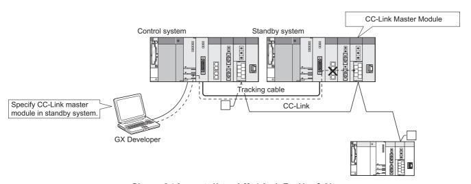
Diagram 6.4 Access to Network Module via Tracking Cable
