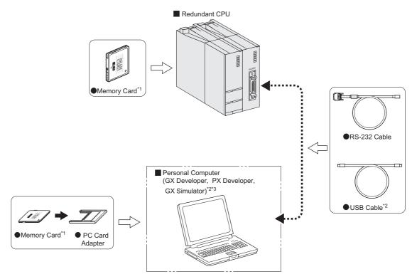
**Diagram 2.11 Peripheral Device Configuration**
