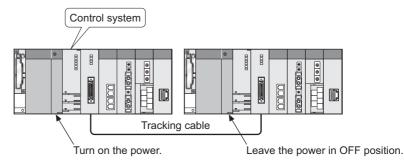
Diagram 5.7 Control System when Only One System Starts Up
