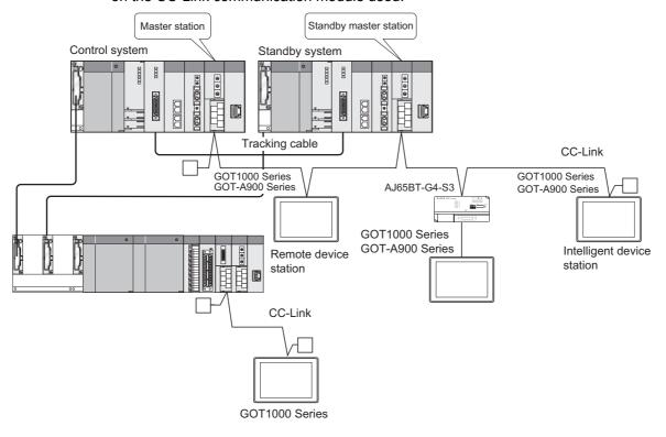
Diagram 6.46 System When Connecting GOTs to CC-Link
