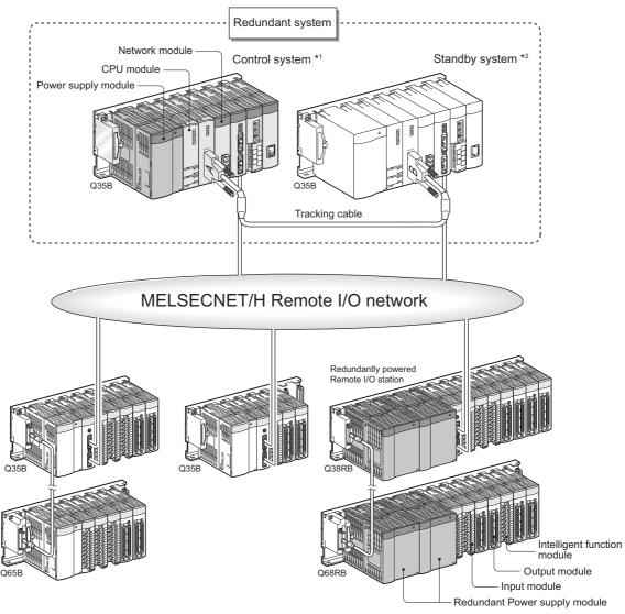
**Diagram 1.1 Configuration Example of Redundant System**
