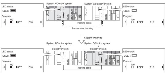
Diagram 7.12 Operation of USER LED When Annunciator (F10) Turns On
