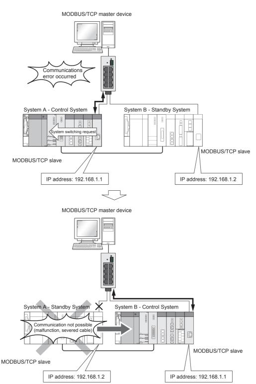
Diagram 6.30 Redundant IP Mode
