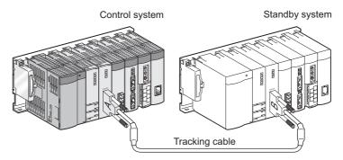
Diagram 1.13 Horizontal Arrangement of Control System and Standby System
