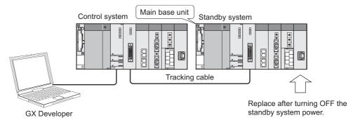
Diagram 8.33 System where Standby System's Main Base Unit Is Replaced
