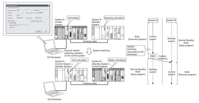
Diagram 5.26 System Switching Operation by GX Developer
