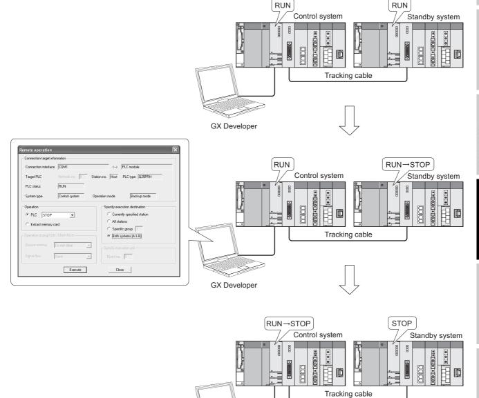
Diagram 5.100 Remote STOP Operation When Both Systems Are Specified
