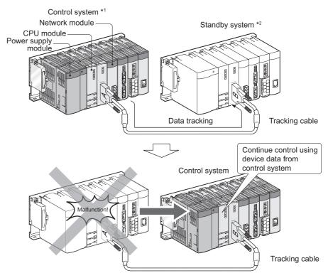
Diagram 1.2 Redundant Configuration of Basic System
